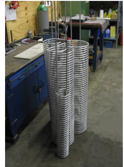
Heiz- /Kühl-Spiralen / Heat- and cooling-spiral DN150 + DN300 /1.4571
