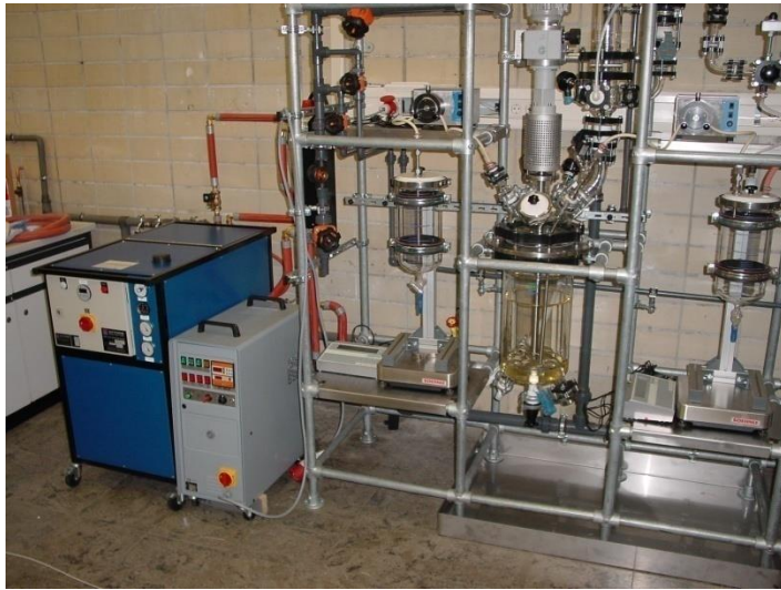
Heiz-+Kühleinheit/ Heating+cooling Unit (-35°C/+150°C)
