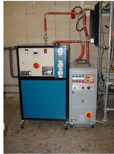
Heiz-+Kühleinheit/ Heating+cooling Unit (-35°C/+150°C)
