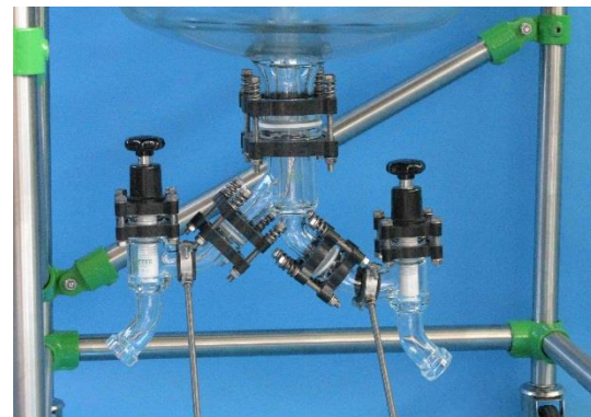
Vak.-/ Ablassventil / Vac-/draine valve
