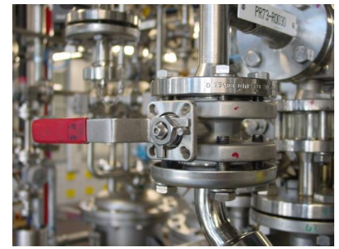
Membran- + Kugelhahn-Armaturen / Membran- + ball valves
