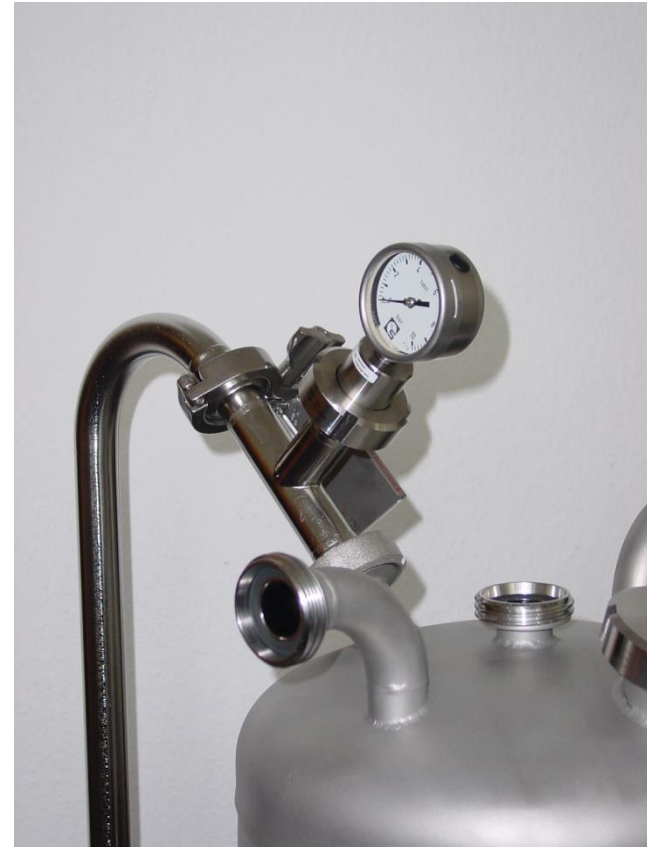
Manometer + Berstscheibe / Pressure gauge + burst disk
