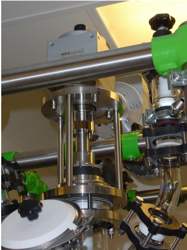
Lagerlaterne m. GRD / Support with mech. seal
