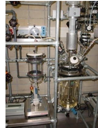
Dosier- Station/ Dosing station
