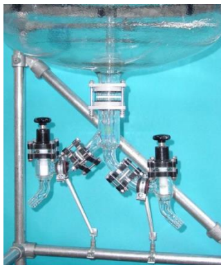
Vak.-+ Ablassventil / Vac.-+ drane valve
