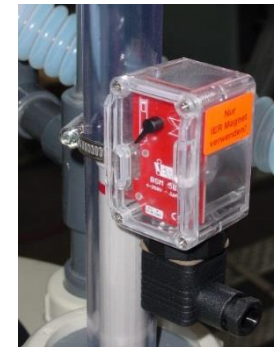
Niveauschalter magn. + bistabil Level switch, magnetic + bistable
