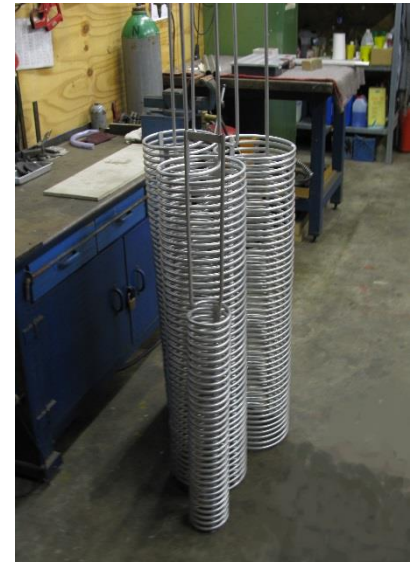
Heiz- /Kühl-Spiralen / Heat- and cooling-spiral DN150 + DN300 /1.4571
