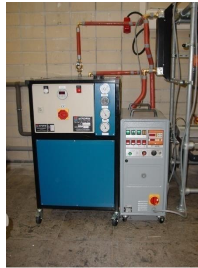
Heiz-+Kühleinheit/ Heating+cooling Unit (-35°C/+150°C)
