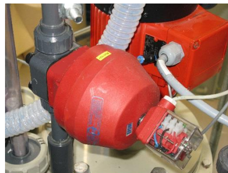
Membrane valve pneumatic + limit switch
