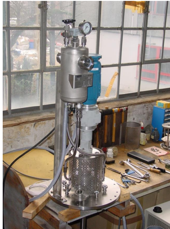
Getr.-Motor m. dw. GRD Gear Motor + double stage seal
