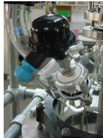
Temperatur- Fühler (PT100)/ Temperature sensor (PT100)
