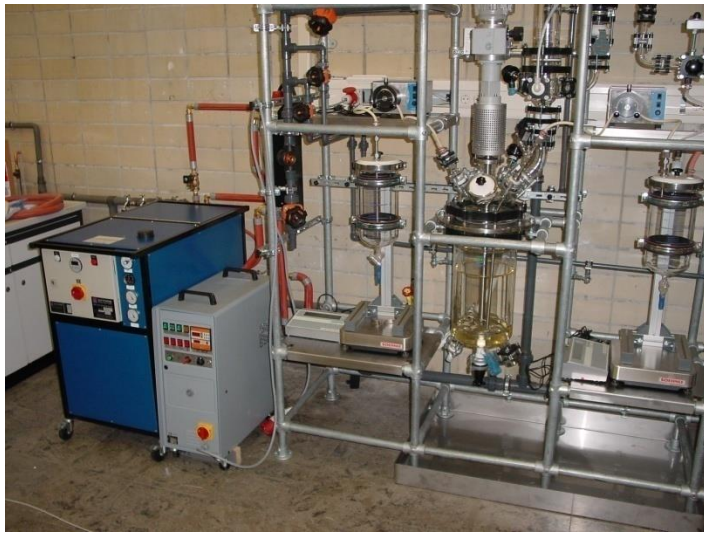
Heiz-+Kühleinheit/ Heating+cooling Unit (-35°C/+150°C)
